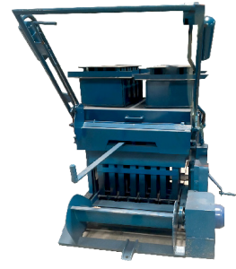
MACHINE A FABRICATION DEBRIQUE BETON
